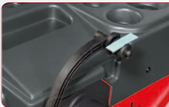
Aludata program that resolves all the problems of balancing aluminium rims. The arm in the central part of the weight holder panel indicates the exact position for application of adhesive weights. The newly developed software enables the balancing machine to recognize and automatically select the Alu program (two internal adhesive weights) with a simple movement of the internal data gauge.
