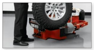
Optional wheel lift eases servicing of large assemblies. Allows for more careful handling of expensive wheels. (20-2045-1)
