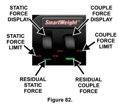
The red-dotted line represents the acceptable amount of force the tire and wheel assembly can have that will not result in a ride problem. Any forces below that line will be shown in green. Any forces that are above that level will be shown in red and indicate an excessive amount of force.
