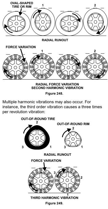
Multiple harmonic vibrations may occur at any harmonic factor, dependant only upon the number of vibration components in each revolution.
