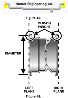
Verify the correct clip-on weight type will be used for the wheel that is being balanced.
