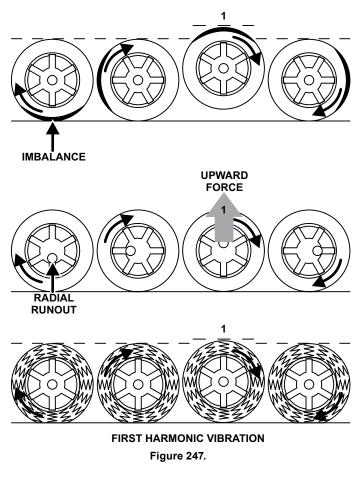
During Forcematching<sup>®</sup>, the first harmonic vibration of the tire is matched opposite of the first harmonic vibration of the rim to decrease the first harmonic vibration of the assembly. This reduces the vibration felt inside of the vehicle.
