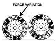
Tire Related Forces are Reveled Only When Testing Under Load Figure 251.
